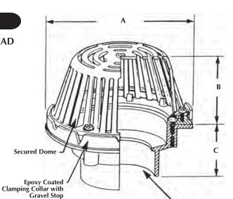
Solvent Weld Connection for 3" or 4" PVC or ABS Sch. 40DWV (Optional SDR 35 Adapter Available)
